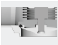
Threaded valve disk, EPDM/FDA or FKM HF seal
